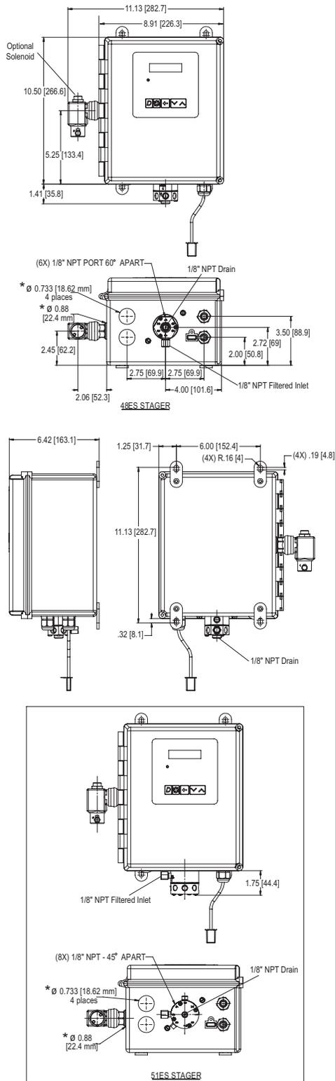
**\*NOTE: Drill as required. These holes will only be drilled at factory if required.**
