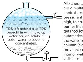
Attached to the boiler are a multitude of safety controls to relieve the pressure if it gets too high, to shut off the burner if the water gets too low or to automatically control the water level. A water column (sight glass) is provided so that the interior water level is visible to the operator.
