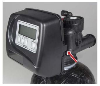
2a. Remove front cover from each control valve. Pull out on each covers release tabs located on each side of the cover and pull cover off.
