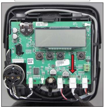
10. Make sure all wires are connected to proper PC Board connections before programming.
