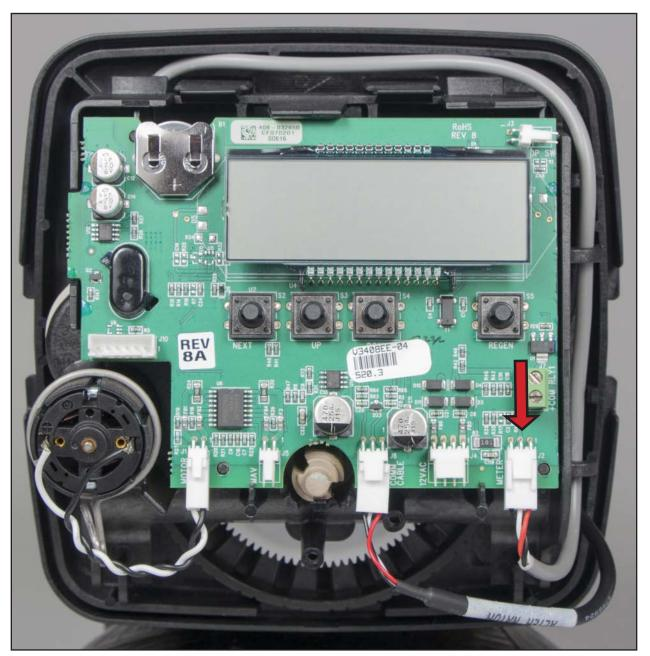
9. **SINGLE METER APPLICATIONS:** Bring meter cable through knockout hole with interconnect cable and connect the 15' water meter cable to the three pin connection labeled "METER" on the "ALT b" control valve to make wiring easier. However, the meter can be connected to either "ALT A" or "ALT b". Connect the interconnect cable to the three pin connection labeled "INTERCONNECT CABLE".
