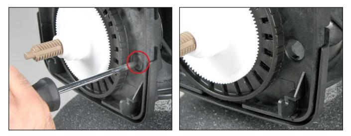
3. Once drive bracket is removed, locate knockout on backplate. You can use a punch or a Phillips screw driver and place it in the center of the knockout circle and tap it with a mild to medium force with a hammer to punch out circle knockout piece.
