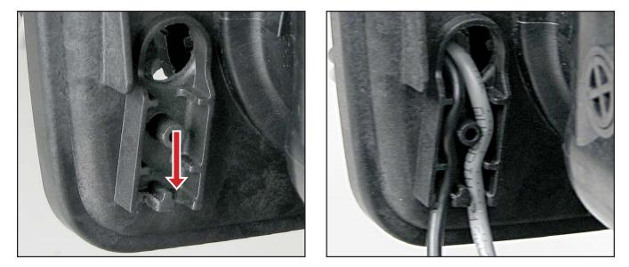
9a. Breakout second tab of "ALT b" strain relief on the backside of the backplate to allow the water meter cable to be weaved through.
