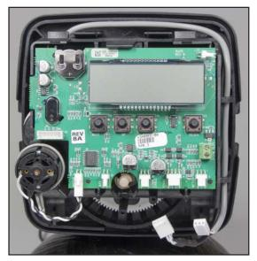
2b. Disconnect power and meter cables from each PC Board.
