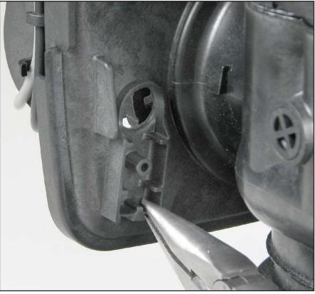
**NOTE:** Since two extra cables need to come to control valve "ALT A" you will need to take pliers and break out the tabs at the bottom of the strain relief on the backside of the backplate.
