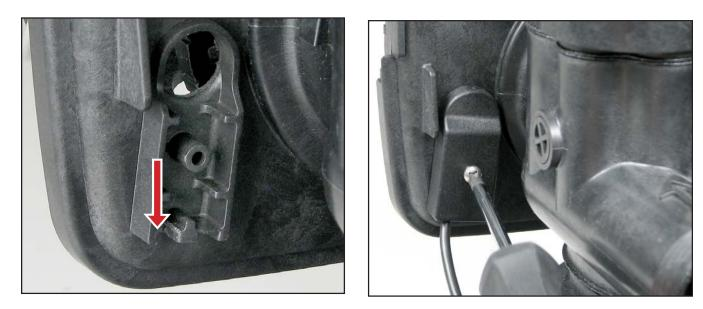
8. On the backside of "ALT b" you will need to breakout only one tab at the bottom of the strain relief for 1" and 1.25" control valves. This will allow to weave the interconnect cable down through the strain relief so you can install and fasten the strain relief cover over the top of the strain relief. See step 9 (pg. 9) for 1.5" and 2" control valves.
